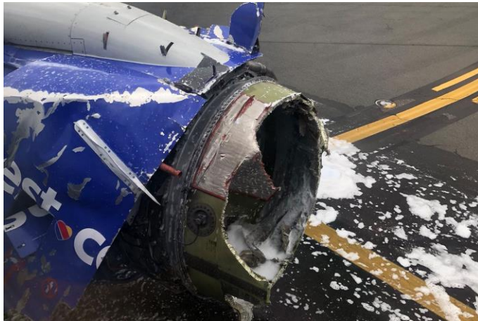
Fatigue failure of turbine blade 1 person killed
